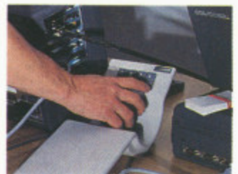
The Spaceball is just one of the control devices accepted by the Sense8 system. Useful for VR exploration, it's a 6D unit, giving control over X,Y,Z co-ordinates and pitch, roll, and yaw
